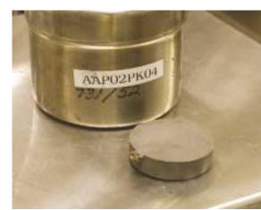
lifetimes in the manifestation of aging effects on weapon design parameters and component function, according to the researchers. The casting yielded nine enriched plutonium "cookies," one of which is shown here. The thickness of this miniature ingot duplicates the thickness of the Rocky Flats ingots, giving researchers a good simulant for the next stage of processing: rolling the ingot into a sheet.
