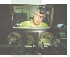
Chris Trujillo of the Nuclear Materials Science Group (NMT-16) machines a Kolsky test specimen. A nonwater-based coolant is used to flood the specimen during machining. Flooding ensures that the sample is not overheated during the machining process, avoiding the introduction of nonaging-related artifacts into the plutonium sample.
